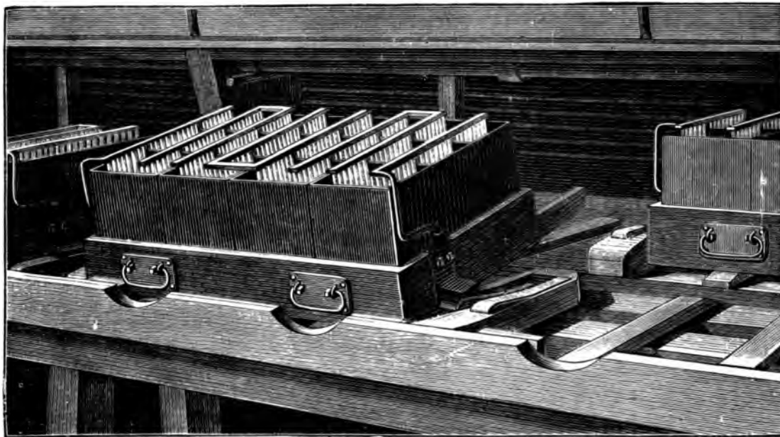
FIG. 2.—THE JULIEN ACCUMULATORS IN STREET CAR SERVICE.
